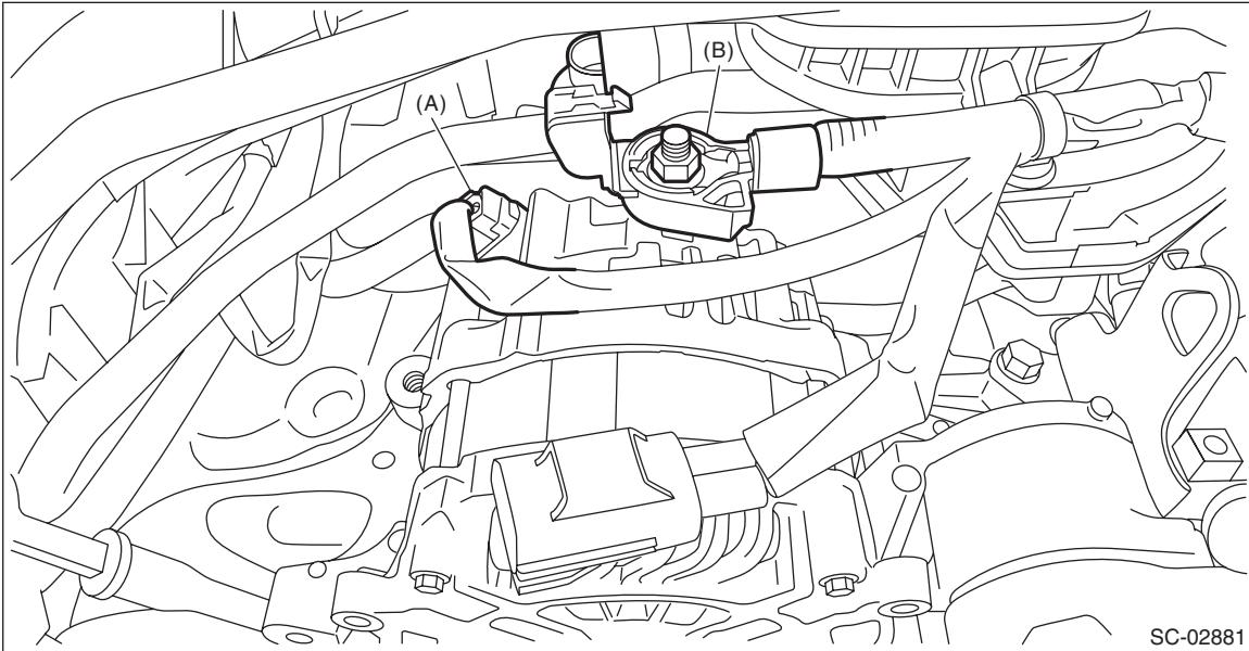
7) Remove the generator from the generator bracket.
