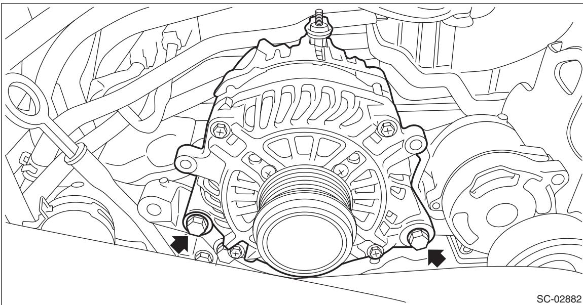
8) Remove the V-belt tensioner. <Ref. to ME(w/o STI)-79, V-BELT TENSIONER ASSEMBLY, REMOVAL, V-belt.>
