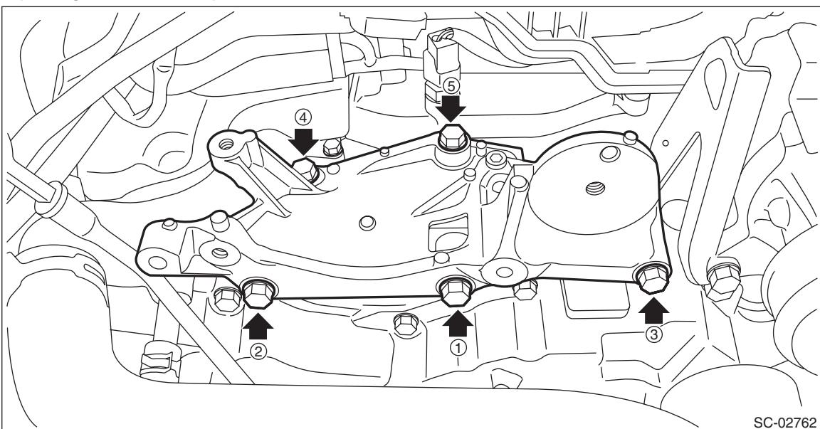
2) Install the V-belt tensioner. <Ref. to ME(w/o STI)-82, V-BELT TENSIONER ASSEMBLY, INSTALLATION, V-belt.>
