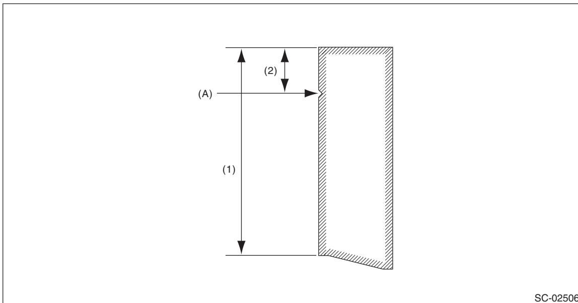
2) Check that there is appropriate pressure on the brush spring. Using a spring pressure indicator, push the brush into the brush holder until its tip protrudes 2 mm (0.0787 in). Then measure the pressure of brush spring. If the pressure is 1.7 N (173 gf, 6.11 ozf) or less, replace the brush spring. 4.1 — 5.3 N (418 — 540 gf, 14.75 — 19.06 ozf) pressure is required on the new spring.
